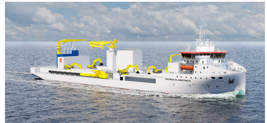
George W. Goethals will install rock around the foundations of wind turbines and subsea cables, mainly in the North Sea and Southeast Asia.
